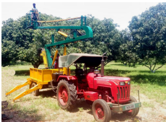
Fig. 1. View of the tractor-mounted hydraulically operated ladder
